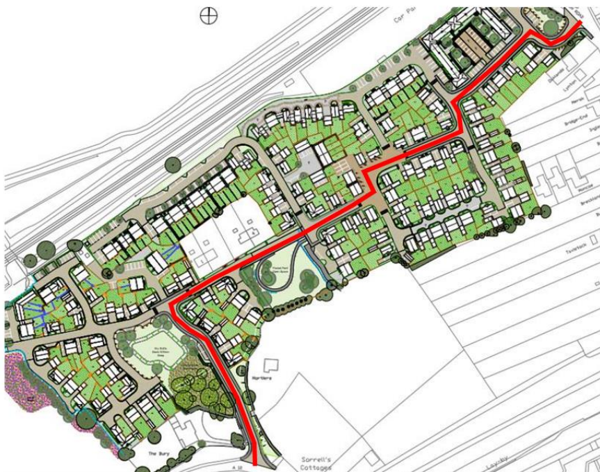
Plate 5.10 Temporary through route
